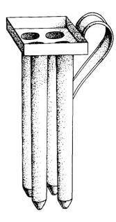
Figure 6. Candle mould. The candle mould was a tubular device with one end narrowed to a conical shape through which the wick was inserted and held taut while the molten fuel was poured into the open end. Most candle moulds were made in tinplate and were generally made in multiples of four, six, eight, or more. A plate across the top held the individual moulds together and also acted as a receptacle for the surplus fuel during the pouring process. Many multiple moulds also had a base plate.
