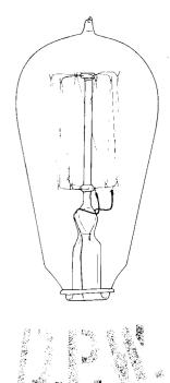
Figure 76. Incandescent lamp and customer mark (1U5A1-21). Height: 12.0 cm (without base). The single wire filament forms a cage, fastened by numerous metallic supports to a central glass tube extending the bulb. Composition: probably tungsten or tantalium. Clear bulb. Approximate date: first quarter of the 20th century. The bulb shows, engraved in acid, the initials DPW, likely those of the client, the Department of Public Works. General use impossible to determine. (Drawing by D. Kappler.)
