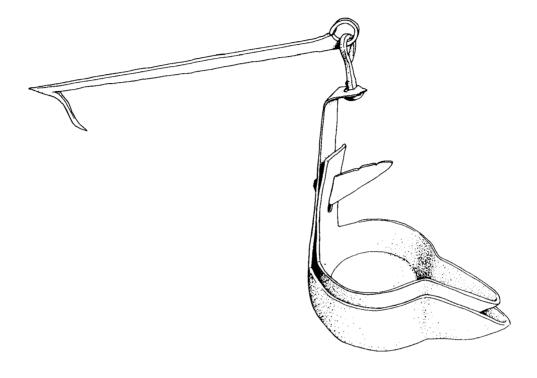
Figure 29. Pan lamp. The illustration depicts the type most frequently encountered, made from forged iron, with a hanging bracket. A drip pan is suspended from the hanger by a swivel device and bears a grooved hook from which the fuel pan is hung. The fuel pan is designed with a broad deep channel for the wick, matched below in the drip pan to catch the unconsumed fuel. The grooved hook allows the fuel pan to be adjusted according to the level of the fuel. (Drawing by D. Kappler.)
