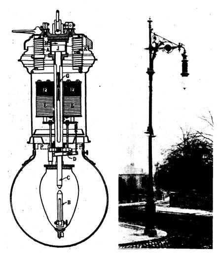
Figure 70. Arc lamp. (a) Diagram. (The Electrician, Vol. 54, No. 3 (1904), p. 100.) (b) Photograph. (The Electrician, Vol. 52, No. 3 (1903), p. 88.)
