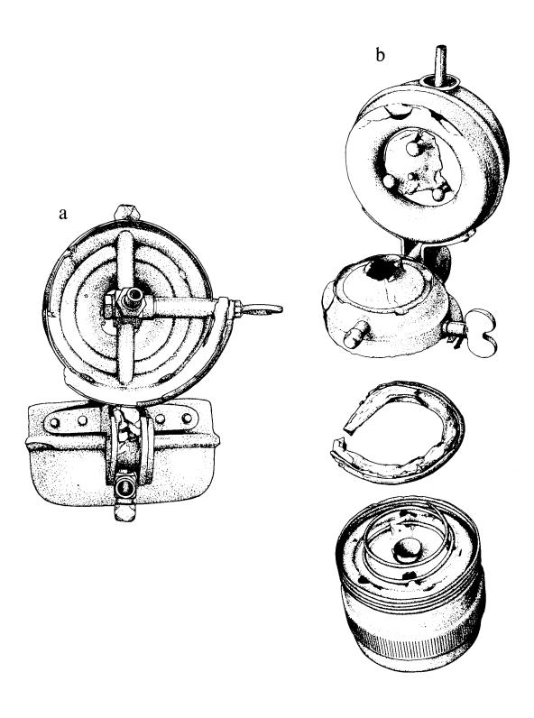
Figure 68. Acetylene lamp for a bicycle. (a) View of the bottom of the cover. (b) Blown-up view. (Drawings by D. Kappler.)
