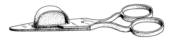
Figure 8. Candlesnuffer. Candlesnuffers worked in a scissor-like motion to trim the charred wicks of candles and lamps. The upper blade bore a vertical plate which forced the charred cuttings into a box mounted on the lower blade.
